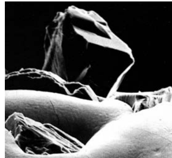
Diamond grinders: The surfaces of industrial diamonds are more regular. Therefore a somewhat coarser graining can be selected (SEM image).
