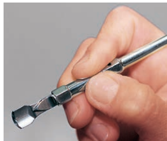
Holding the hollow blade like a pen when working supports the user's fine motor function and allows particularly sensitive filigree work.
