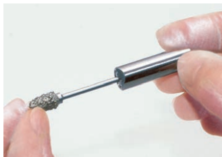
Position the dust protection ring approx. 5 mm from the lower end of the grinder shaft. Push the grinder with the dust protection O ring into the hand piece to the stop.
