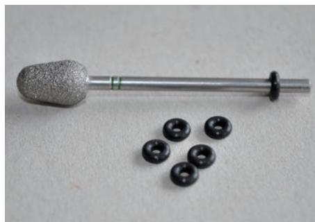
Position the dust protection ring approx. 5 mm from the lower end of the grinder shaft. Push the grinder with the dust protection O ring into the hand piece to the stop.
