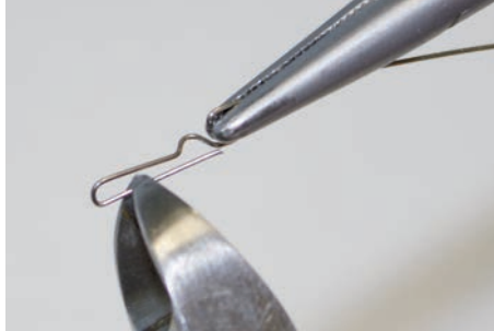
2. Shortening the bent brace ends
