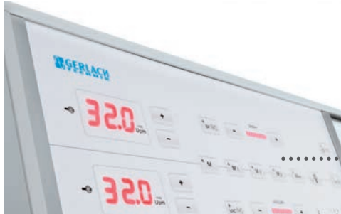
User-friendly, easily cleaned key pad, 25° incline
